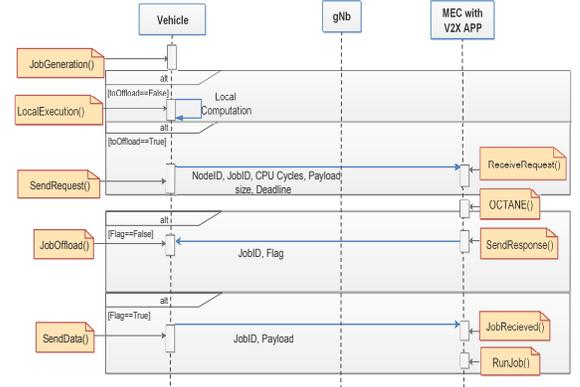
Fig. 2: Sequence Diagram of UdpOffloading Application.
